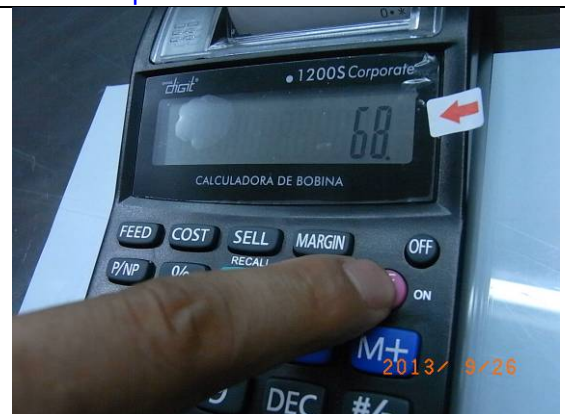
Major defects- Malfunction(can not clear to zero)
