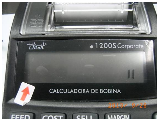
Major defects- Malfunction(no information on LCD screen)
