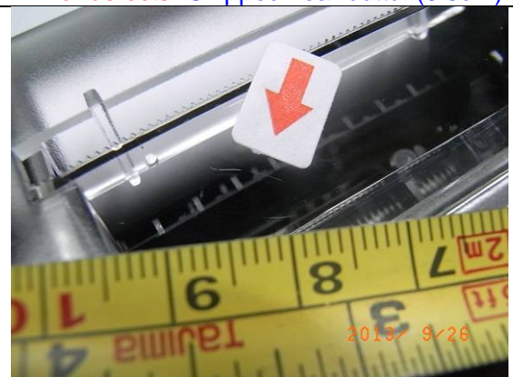
Minor defects- Scratched mark on clear cover(1.3cm/1.0cm)
