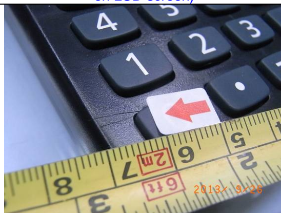
Minor defects- Flash in buttun(1.2cm)
