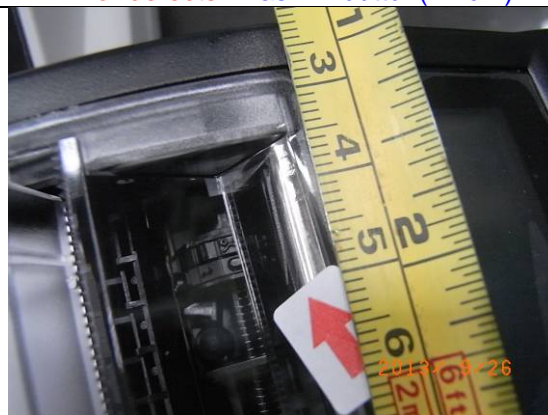
Minor defects- Scratched mark on clear cover(1.3cm/1.0cm)
