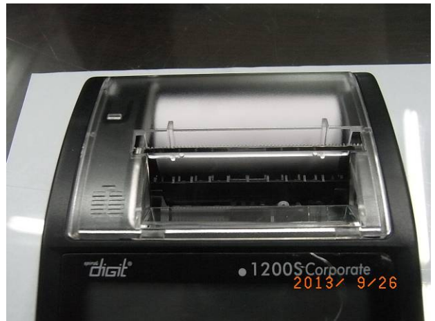
defect sample (the cover can't open)
