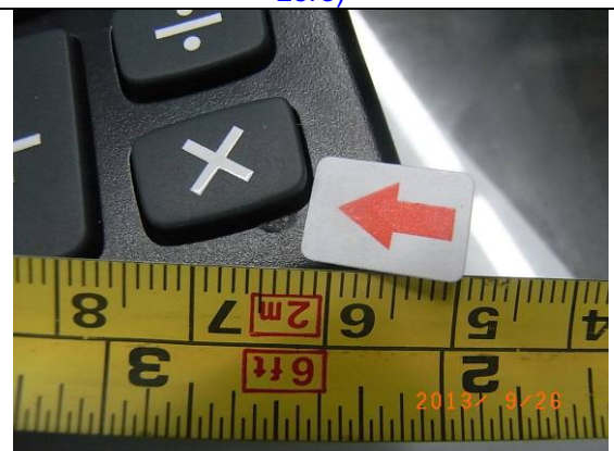
Minor defects- Chipped near buttun(0.3cm)
