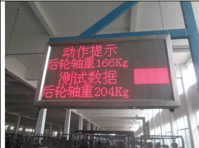
Rear axle weight shown on factory test equipment
