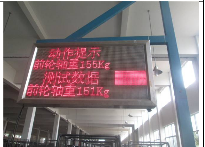
Front axle weight shown on factory test equipment
