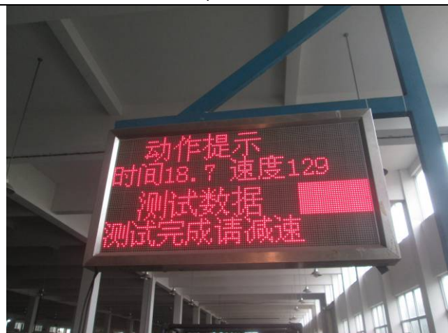
Max speed check shown on factory test equipment
