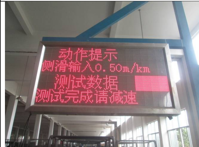
Sideslip test shown on factory test equipment
