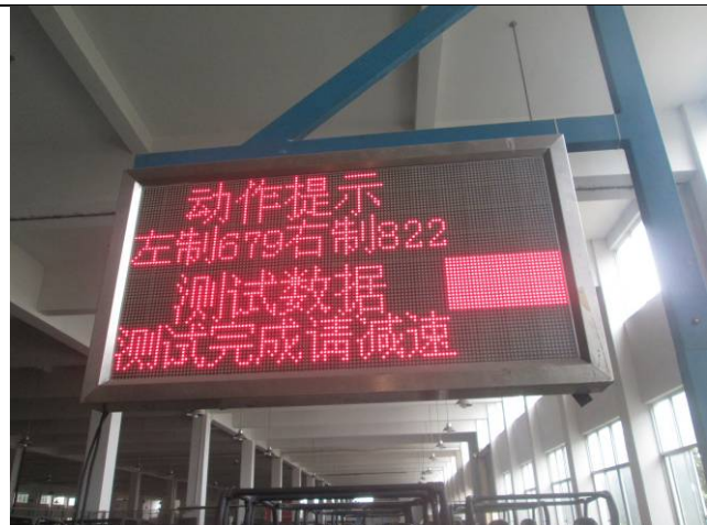
Brake function check shown on factory test equipment
