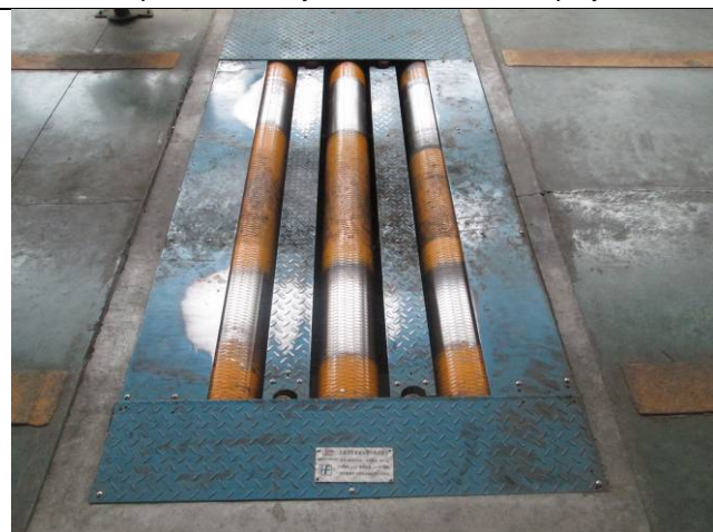
Max speed check & Speed accuracy check test equipment
