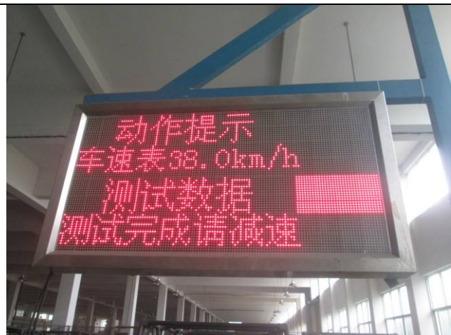
Speed accuracy check shown on factory test equipment
