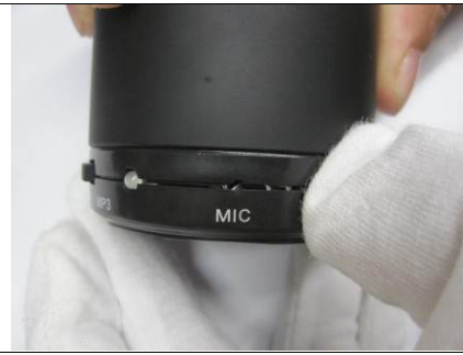
Photo 35) Gap on the product due to loosen screw.
